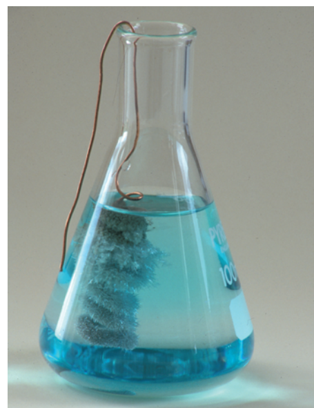
Figure 8.10 Displacing silver from silver nitrate solution.
